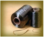
Fig. 1. Bobbins of basalt roving [12]
